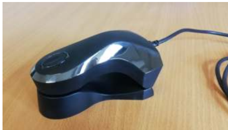
Fig. 1. OligoCheck spectrophotometric sensor unit on its stand. Top: button to used to initiate scanning; bottom (not visible, hidden in stand): sensor's head.
